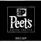
080' ROUTED ALUM FACE-÷ ALUM CABINET FRAME-1/2" THICK ROPT LOGO FIELD WITH 1ST SURFACE TRANSLUCENT VINYL 1A" CLEAR AGRYLIC COFFEE CUP W/ OPAQUE VINYL DECORATION . TOGGLE DISCONNECT SWITCH 1/2" CLEAR ACRYLIC ROPT PEETS WHITE PLEX BACKING FOR ROST DROP SHADOWS & BORDER 1ST SURFACE VINYL COFFEE AND TEA GRAPHICS GE 7100K WHITE EDGE-STRIP LED 4-1/2"
