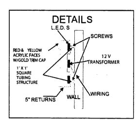
27" X 18' CHANNEL LETTERS 5" RETURNS TO BE ATTACHED TO WALL ON 1' X1' SQUARE TUBING STRUCTURE
