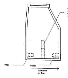
Concrete supported stainless steel weir wall with 60 degree v-notch weir
