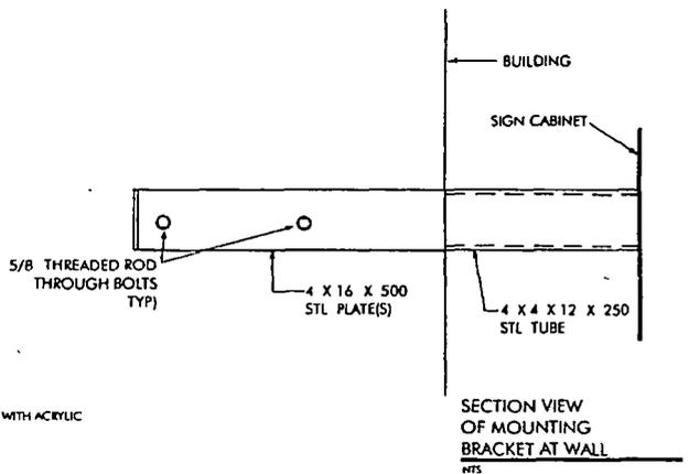
**SECTION VIEW OF MOUNTING BRACKET AT WALL**
