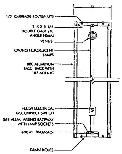
(1) DOUBLE FACED INTERNALLY ILLUMINATED WALL CABINET WITH ROUTED OUT TEXT & LOGO BACKED WITH ACRYLIC
