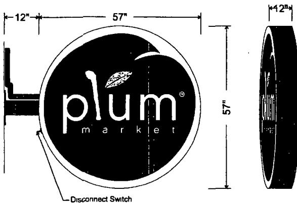
12" deep fabricated aluminum blade sign, .090 Aluminum return with .1875 #7328 translucent white acrylic faces, with respective color vinyl graphics applied 1" std white trimcap Returns painted PMS 222C Steel structure included for mounting to 5" x 5" x 3/16" tube
