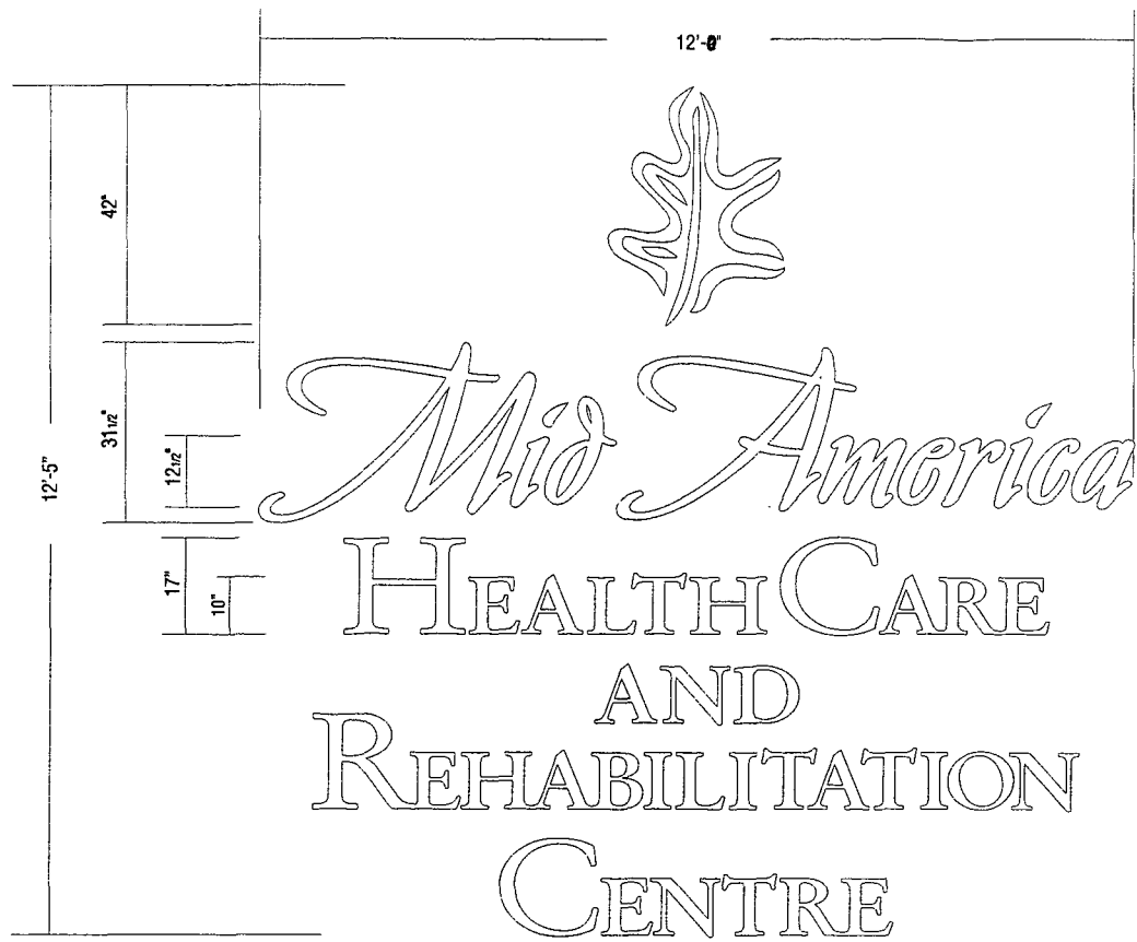
(A) INDIVIDUAL FCO LETTERS 1/2" = 1'-0" 1" THICK FCO LETTERS / WHITE POLYURETHANE FINISH STUD MOUNTED / 1" SPACERS
