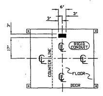
NOTE: PROVIDE 120/240V. 10-3' WIRE SERVICE WITH GROUND. SERVICE ENTRANCE/ANCHOR BOLT LAYOUT
