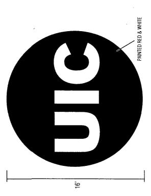
(1) 16" DIA. x 6"(D) ALJIMINUM FACED NON-ILLUM. CHANNEL SIGN, PAINTED RED & WHITE - PIN MOUNTED ON EXTERIOR WALL
