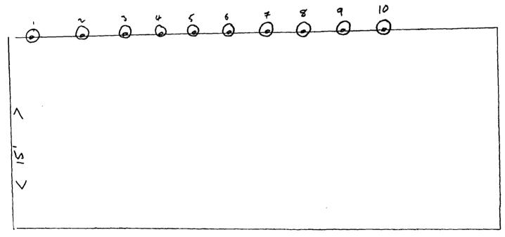
Note: Each light Fixture is .5' wide and hangs From the wall on conduit 1s reet long. There are ten lights in total all of which are hung 15' Above the Grade
