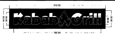
Front-Lit, Plex-Face Channel Letters w/ LED, Raceway Mounted • Front View SCALE 0/0' = 1'0' For Production / For Presentation
