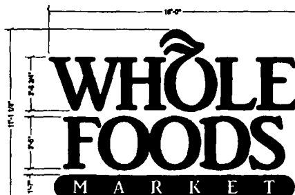
(C) ONE(1) I.L.D. ILLUMINATED CHANNEL LETTER DISPLAY, RACEWAY MOUNTED • FRONT VIEW SCALE: 1/4"=1"
