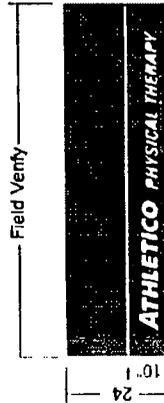
Aluminum frame w/ Sunbrella fabric with blue to match PMS 2945C w/1st surface applied white vinyl graphics, attached to exterior wall using z-clips into mortar face
