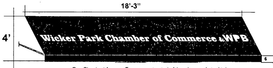
One Standard Awning Frame constructed of 1 galvanized steel tube
