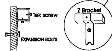
Awning frames can easily be mounted with these bracket.
