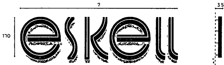
QTY (1) 2 thick fabricated aluminum letters. Back lit with warm white LED's Weight 100 lbs Area 13 sq ft
