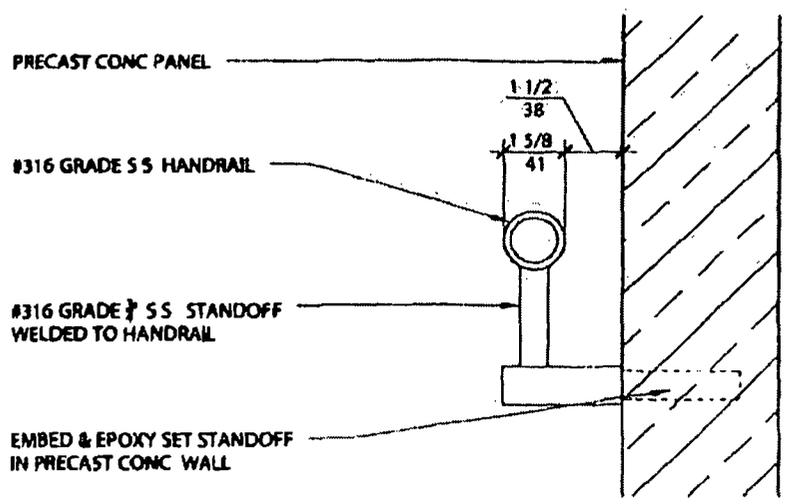
**HANDRAIL DETAIL @ PRECAST CONCRETE WALL TYP.**
