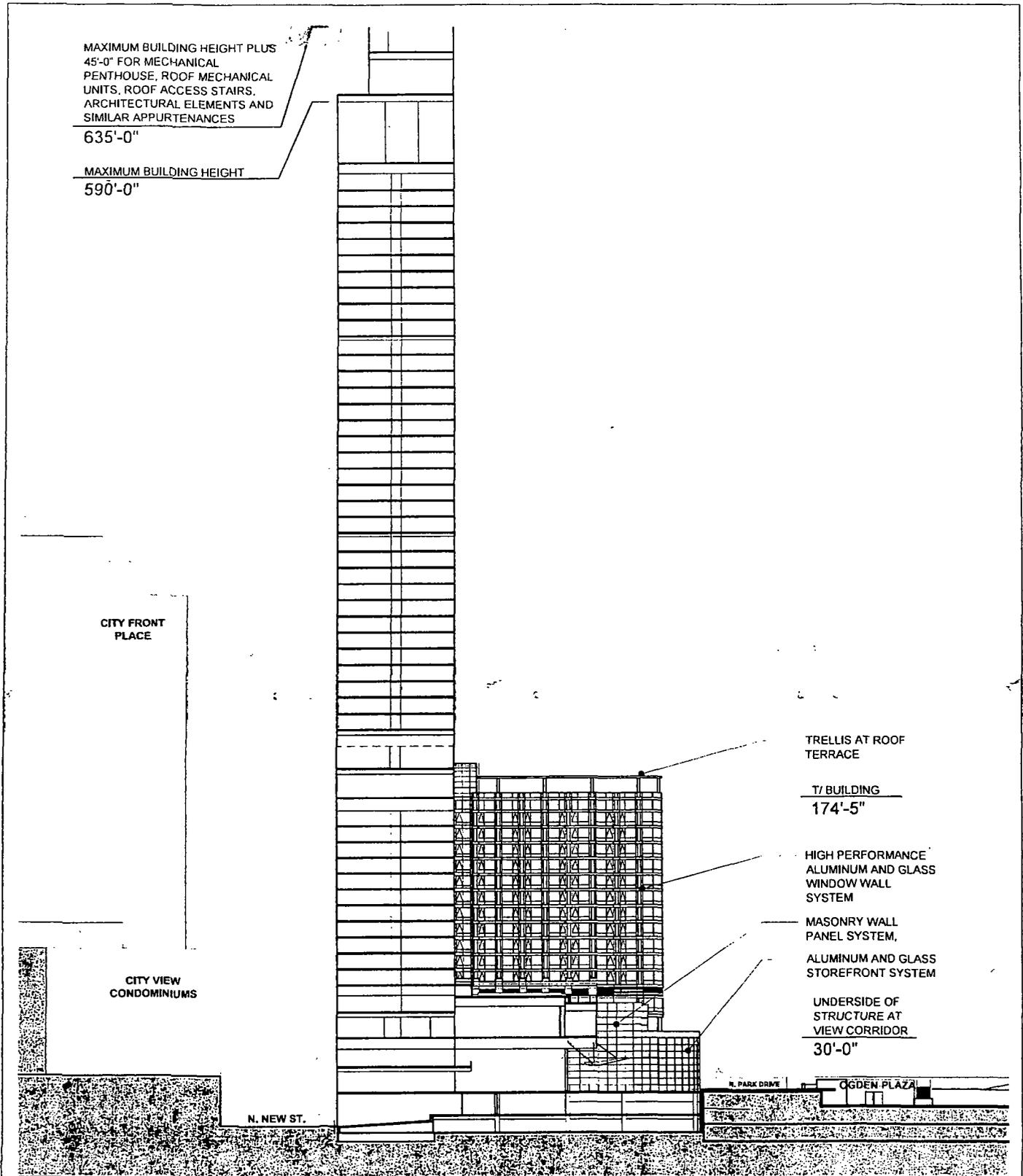
**OVERALL SECTION A AND PARTIAL NORTH ELEVATION**
