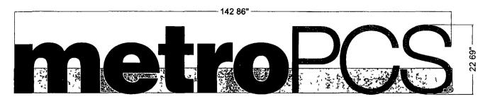
Front-Lit, Plex-Face Channel Letters w/ LED, Raceway Mounted @ Front View SCALE 0/0 = 1'0" @ For Production / For Presentation
