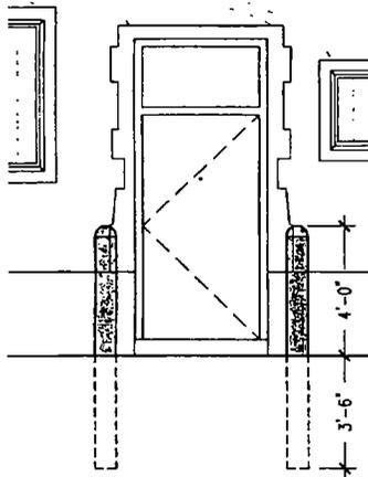
**2 Bollard Elevation**
