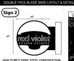
SIGN TO BE 5" DEEP, STEEL CONSTRUCTION INTERNALLY ILLUMINATED BY LED LIGHT WITH LOGO (REVERSE LIGHTING) WILL MOUNTED ON THE ALUMINUM PANEL.
