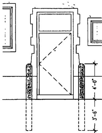
2 Bollard Elevation
