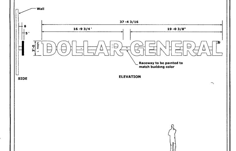
3/16" Yellow #2037 acrylic face with **Mill Coated Matte Black returns** To be mounted to Signcomp 8" raceway Illuminated with AgiLight White LED's
