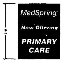
(C) ONE(1) FIRST SURFACE WINDOW VINYL GRAPHIC SCALE: 1/4"=1 BLUE & WHITE FIRST SURFACE CONTROL TAC VINYL TO MATCH EXISTING INTENSE BLUE #127
