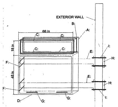
A: 18" X 66" X 28" DOUBLE FACE SIGN CABINET B: 2" X 2" X 3/16" GALVANIZED ANGLE IRON FRAME WORK. WELDED IN ALL CORNERS WITH 2" X 2" X 3/16" ANGLE
