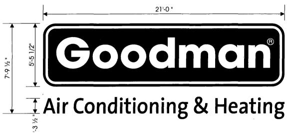
(1) COMPLETE S/F INTERNALLY ILLUMINATED CABINET SIGN, WITH FLEX FACE. FIRST SURFACE DECORATION. THE CABINET DEPTH IS TO BE 10". THE RETAINER IS FIGURED FOR 2 3/4". THE SIGN IS TO BE UL LISTED WITH A SERVICE SWITCH INSTALLED. THE SIGN IS TO BE FLUSH MOUNTED TO WALL.
