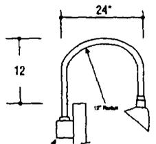
3/4" SINGLE REFLECTOR GOOSENECK WALL BRACKET W/ RIGID CONDUIT & CAST WALL PLATE. MOUNTS TO RACEWAY BOX MOUNTED TO BACK OF SIGN (BY HEATH)
