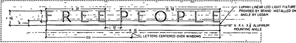
NOTE: THIS SIGN IS INTENDED TO BE INSTALLED IN ACCORDANCE WITH THE REQUIREMENTS OF ARTICLE 600 OF THE NATIONAL ELECTRICAL CODE AND/OR OTHER APPLICABLE LOCAL CODES. THIS INCLUDES PROPER GROUNDING AND BONDING OF THE SIGN.
