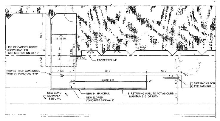
SITE PLAN - SLOPED SIDEWALK & CANOPY SCALE 1/8 = 1 0
