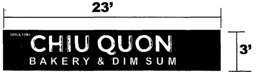
**A** Front & Back L4 Plex Face Channel Letters Self Contained Recessed Mounted w/LED Front View
