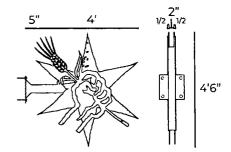
Distressed painted "TAPROOM" on 1/4" dibond backer attached to brick with bults in 4 corners - Illuminated with qty 2 60w/120 v spotlights East Elevation - Sign Area - 8 sq ft - 15 lbs
