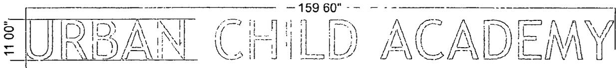
**A** Stainless Steel Fabricated without backs • Stud Mounted • Front View
