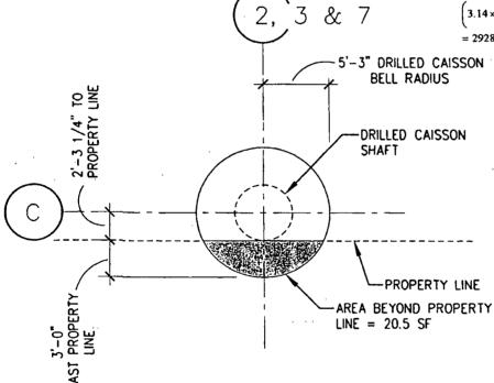
DRILLED CAISSON DC54 @ W. KINZIE ST. (3 TOTAL)
