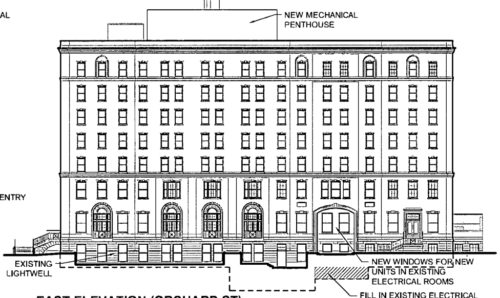
EAST ELEVATION (ORCHARD ST)
