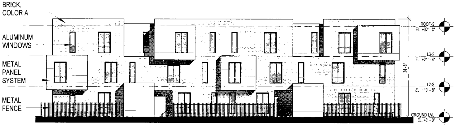
① SOUTH BUILDING - WEST ELEVATION
