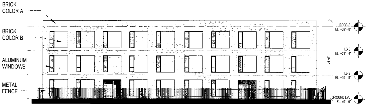
② SOUTH BUILDING - EAST ELEVATION
