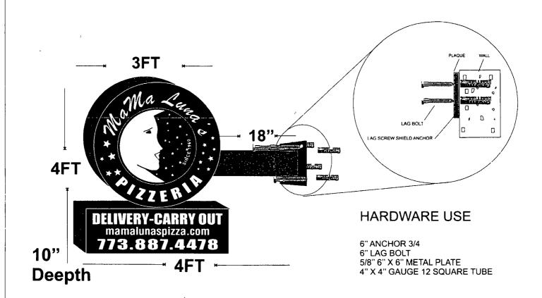
Electrical Sign Light up by Led modules powered by 12Volts Led power supply powered by 110V 2Amps
