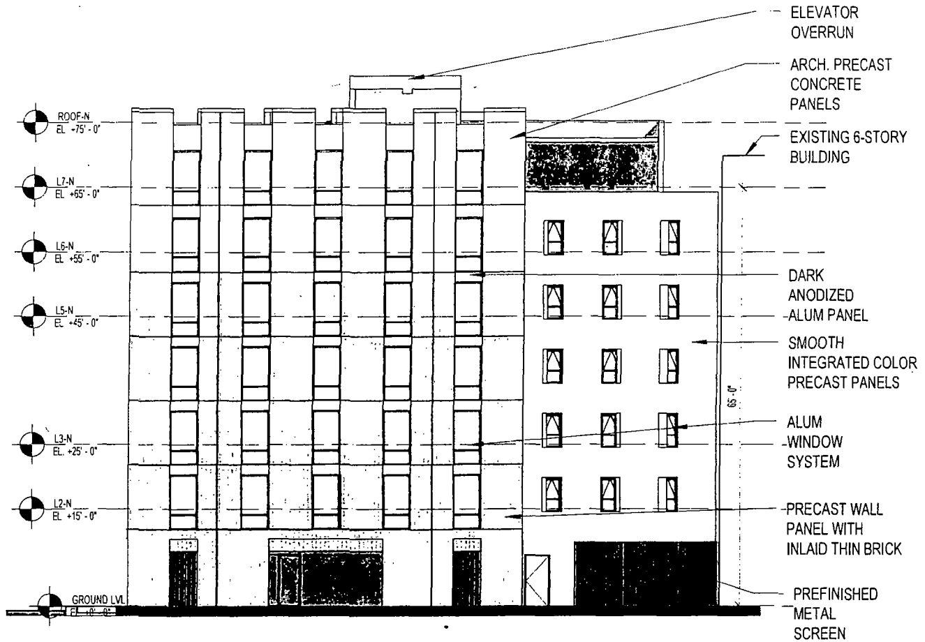
1 NORTH BUILDING - SOUTH ELEVATION
