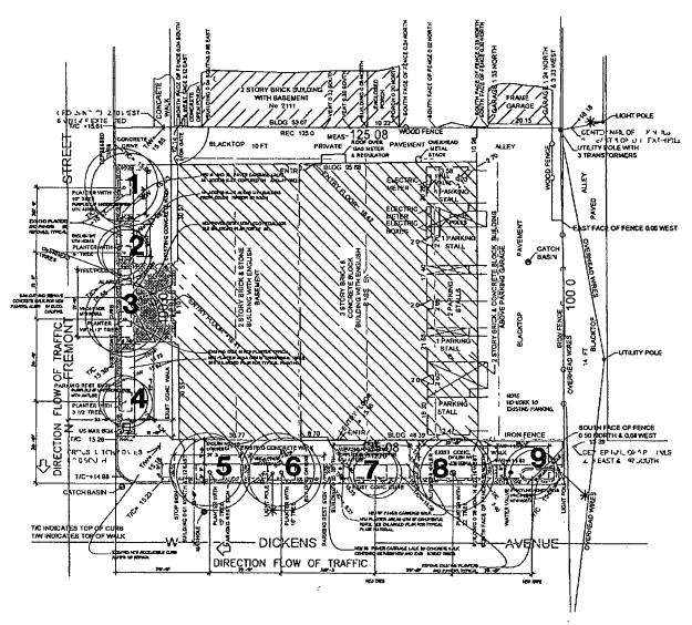
NOTE: CARRIAGE WALK AND BORDER PAVERS SET IN PERMEABLE BED AT GRADE FROM EXISTING STREET CURB TO EXISTING CONCRETE SIDEWALK. EXISTING PAVERS REMOVED TO CREATE LARGER PLANTING BEDS NEW 18 WIDE PAVER CARRIAGE WALK REPLACES LARGER PAVER WALK. 18' HIGH ORNAMENTAL FENCE SET ON INDIVIDUAL PIERS WITHOUT CURB ALL FOUR SIDES.
