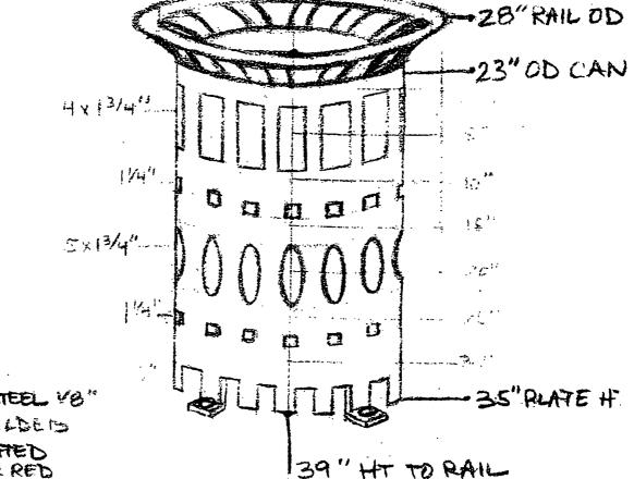
LASER-CUT STEEL VE" RELEDIWELDERS POWDER-CORTED YELLOW DE RED
