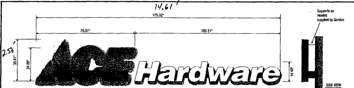
**A** NEW INTERNALLY ILLUMINATED PAN CHANNEL LETTERS SCALE 3/4" = 1'-0"
