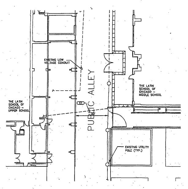
ROUTE (1) 4" RGS CONDUIT FROM EXISTING BOILER ROOM LOCATED AT THE UPPER SCHOOL TO SERVER ROOM LOCATED AT FIRST FLOOR OF THE NEW MIDDLE SCHOOL RUN CONDUIT 24" BELOW GRADE TO ABOVE BASEMENT CEILING AND 90' UP TO SERVER ROOM.
