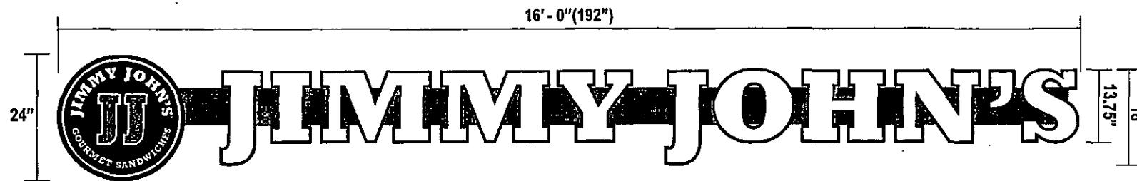
**A** Front-Lit, Plex-Face Channel Letters, Raceway Mounted • Front View
