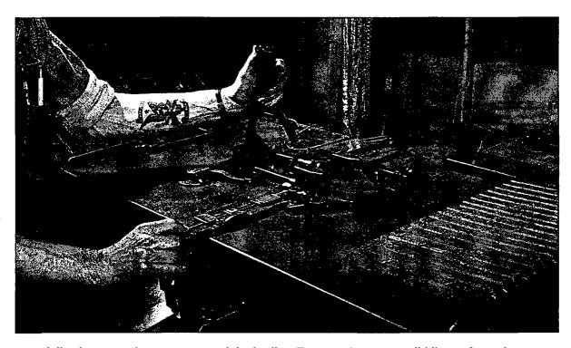
Specialized typograph operators used the Ludlow Typograph to cast solid lines of type from selected matrices arranged in Ludlow casting stick.
