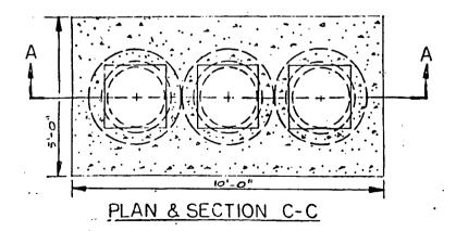
GREASE SEPARATOR SCALE: 1/2 - 1-0"
