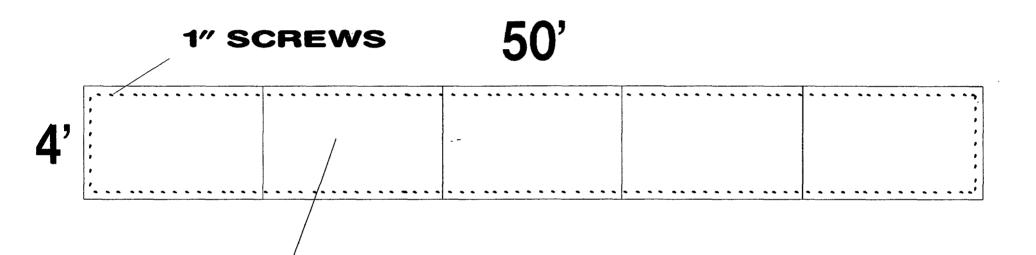
5 (4' X 10') FLAT ALUMINUM .40 INSTALLED AGAINST A WOODEN BACK W/1' SCREW EVERY 6"
