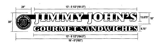
Front-Lit, Plex-Face Channel Letters, Raceway Mounted • Front View SCALE: 3/8" = 1' 0" · For Production / For Presentation
