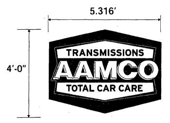
Two 4' x 5.316' Pan Formed Faces and illuminated box sign, Panned & Double Embossed Pan Faces
