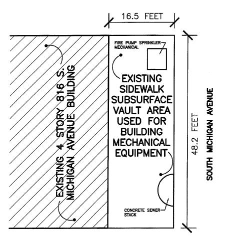
SITE PLAN AT SIDEWALK VAULT AREA USED FOR MECHANICAL EQUIPMENT
