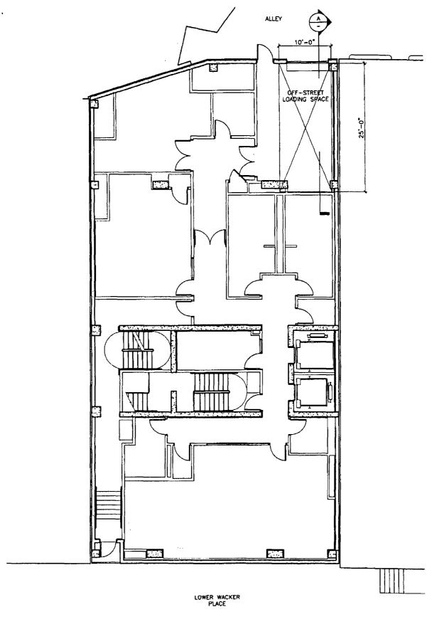
OFF-STREET LOADING - LOWER LEVEL PLAN SCALE: NTS
