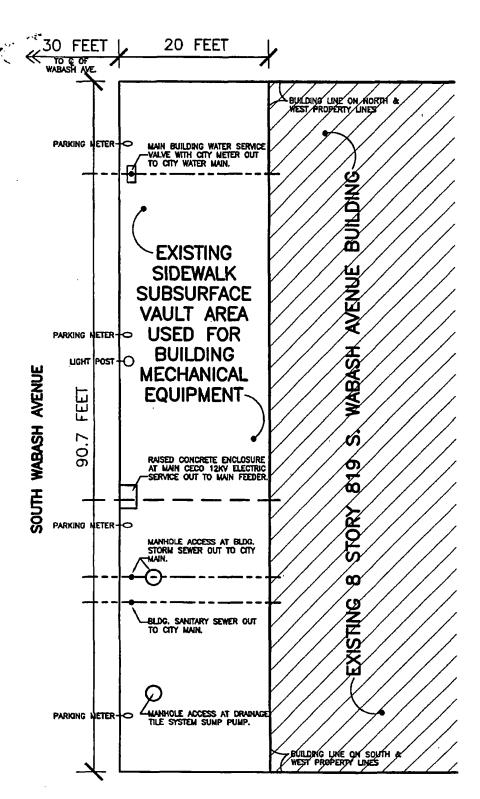
SITE PLAN AT SIDEWALK VAULT AREA USED FOR MECHANICAL EQUIPMENT
