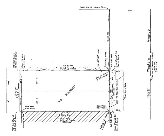
LEGEND conc = concrete R.O.W. = right-of-way rec = record meas = measured pch = porch, N = North
